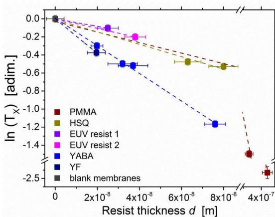
For all samples,  $\ln(T_x)$  varies linearly with  $d$ : **homogenous absorption**. Dashed lines are linear fit, **weighted** on  $\sigma_{I_0}$  and  $\sigma_d$ ; their **slope** gives  $\alpha$ .
