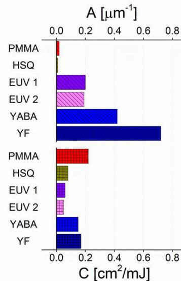
Dill parameters define how the absorption of a photoresist varies after exposure (A), its final value (B) and its rate of change (C).
