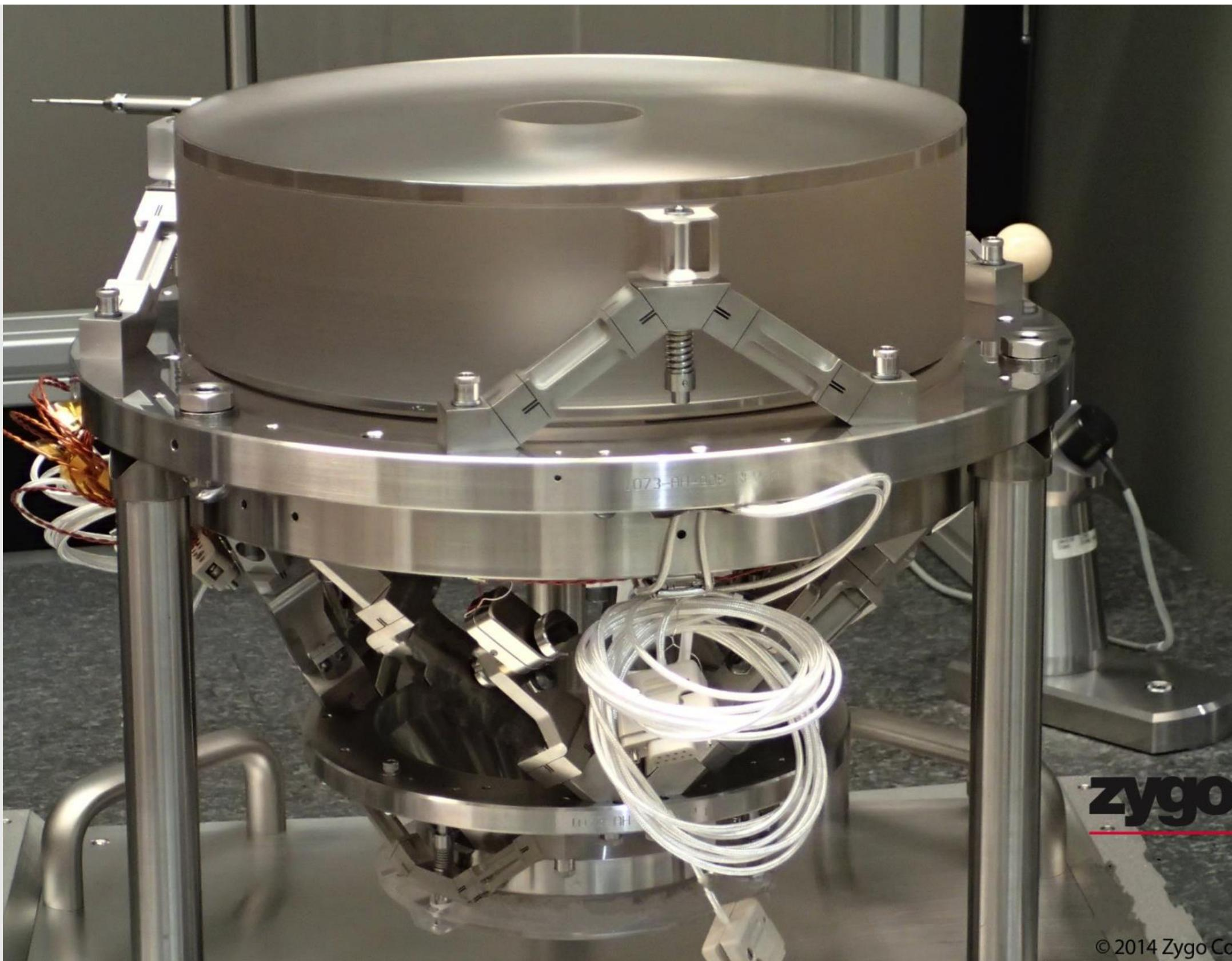
System wavefront error = 0.21 nm at center of field (spec = 0.5 nm)
