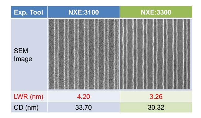
LWR was improved about 20% by NA 0.33, even though the resist film thickness and the reticle were different.
