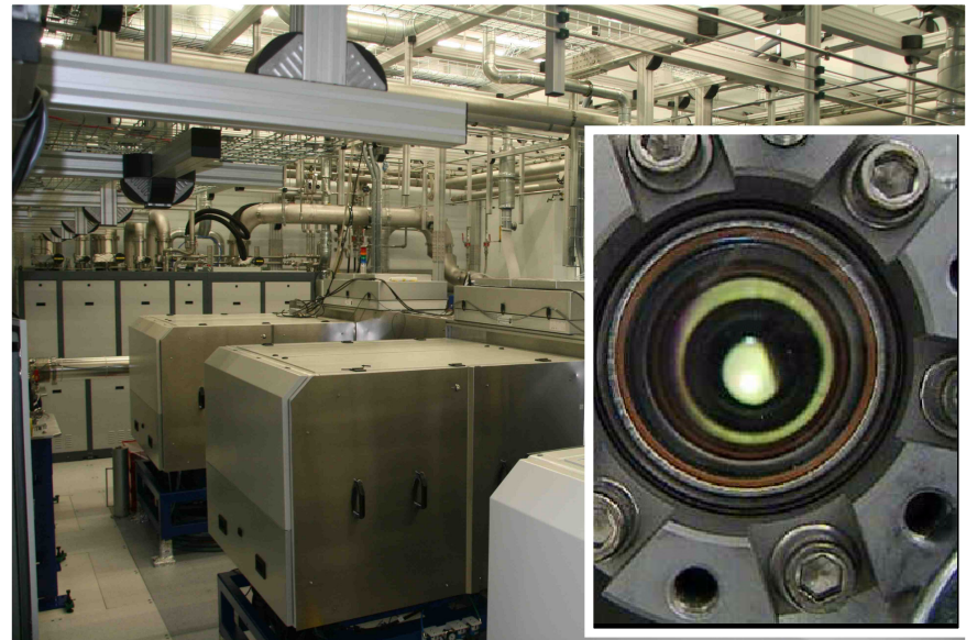
CO 2 Laser amplifiers in subfab
