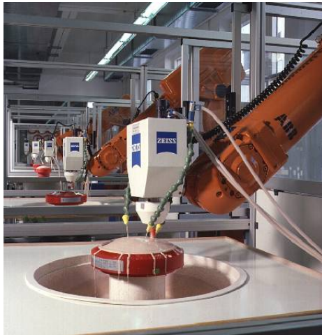
Computer Controlled Polishing for Deterministic Processes
