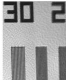
1:1 lines—clearly resolved to 125 nm hp actinic image
