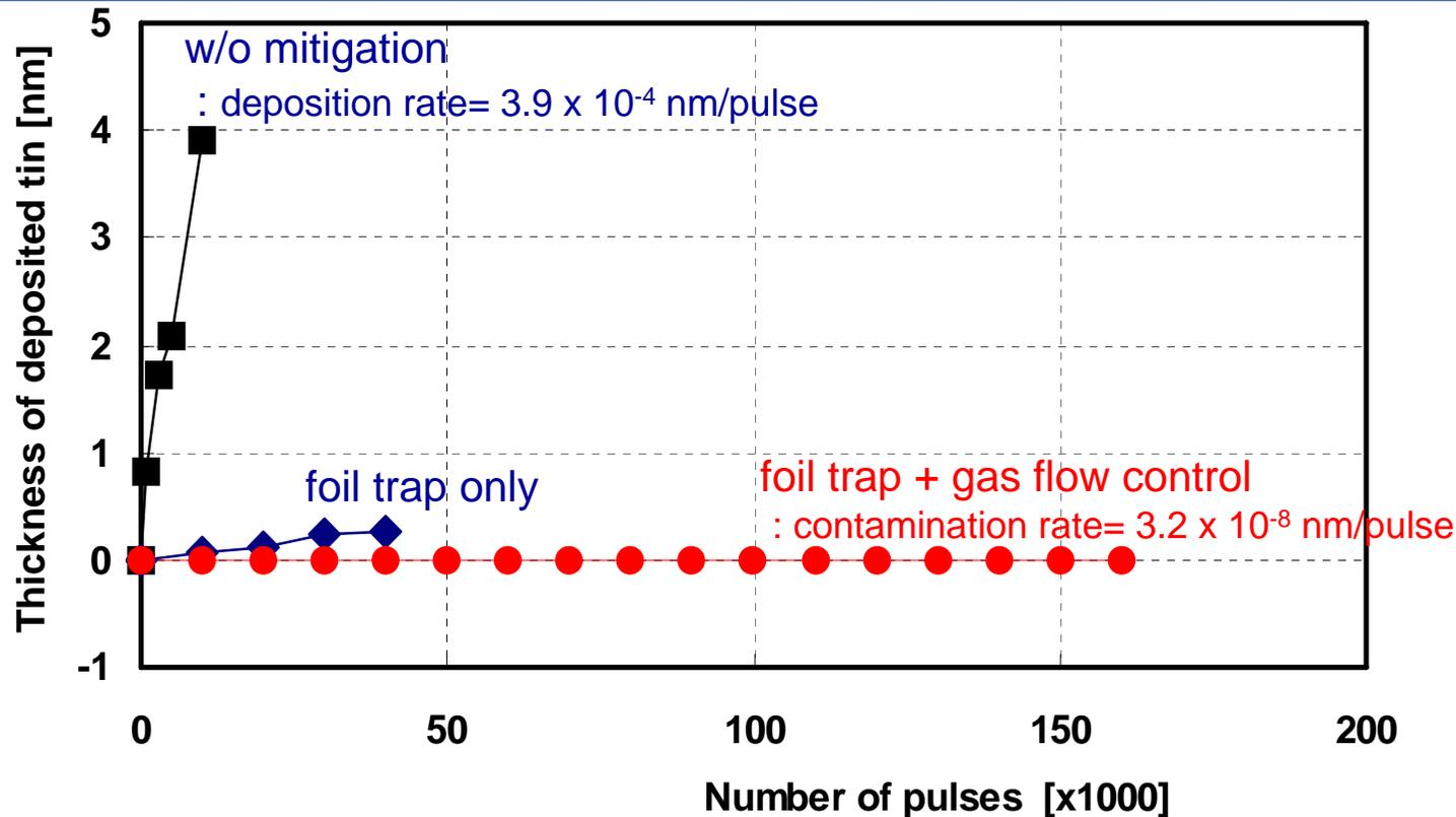
Sn contamination rate was  $1.0 \times 10^{-6}$  nm/pulse with the foil trap. Sn contamination rate was  $3.2 \times 10^{-8}$  nm/pulse with the foil trap and gas flow control. The experimental condition was 1 kHz of pulse repetition rate, 10 sec/set, polished QCM-crystal with Ru layer.
