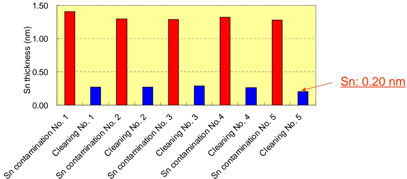
5 times of Sn contamination and Halogen cleaning were continued. Sn contamination was about 1 nm/time. Cleaning rate was 99%/time on average. After 5 cleaning, Sn thickness was 0.20 nm by QCM. The average (5 times) of Sn thickness after cleaning was 0.26 nm. The QCM was polished about 1.0 nm@Ra and was Ru layer. This QCM looked like a sample mirror.
