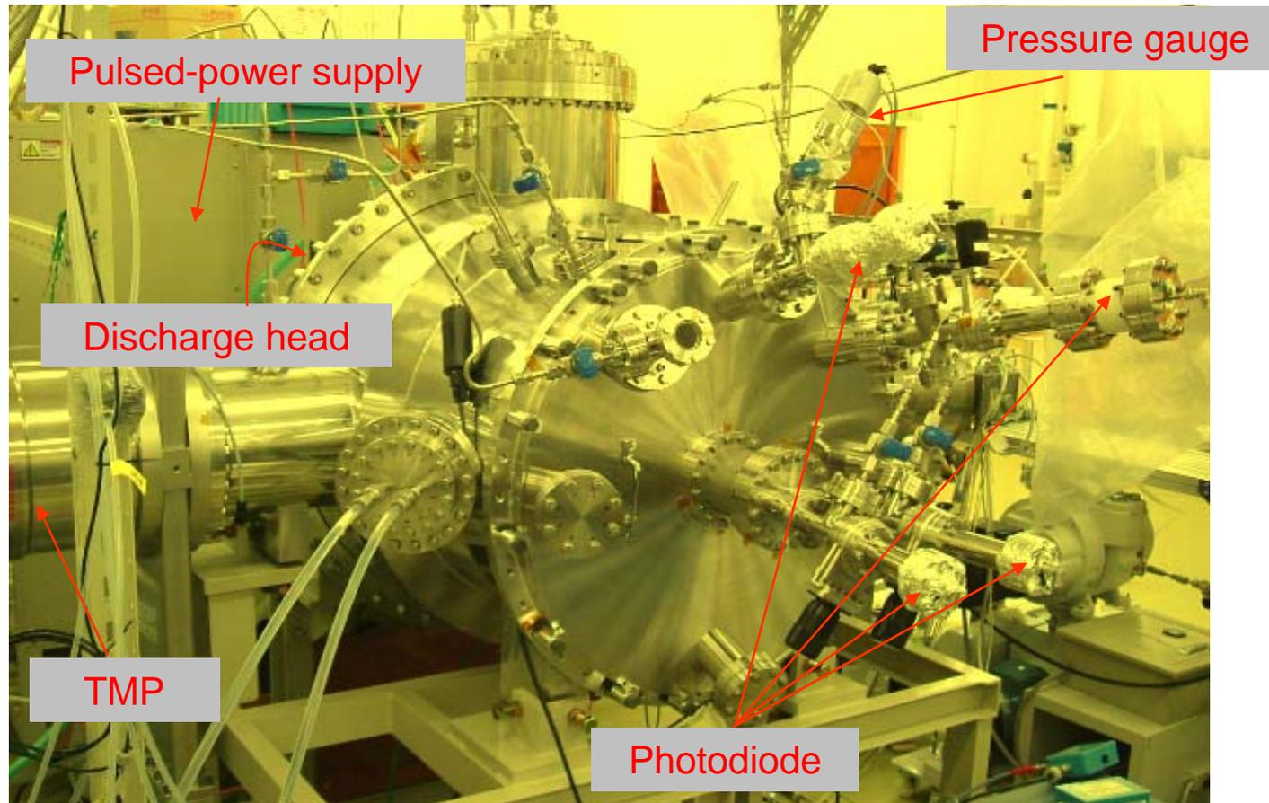
Mirror lifetime measurement chamber and pulse-power supply
