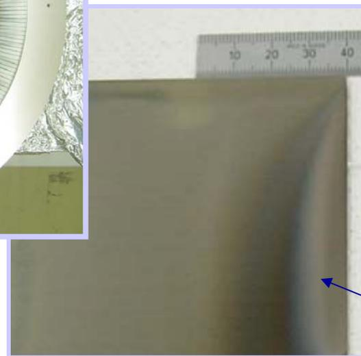
This foil was exposed to about 5 Mshots of pulse. Sn contamination was 30 mm from the side of EUV source.
