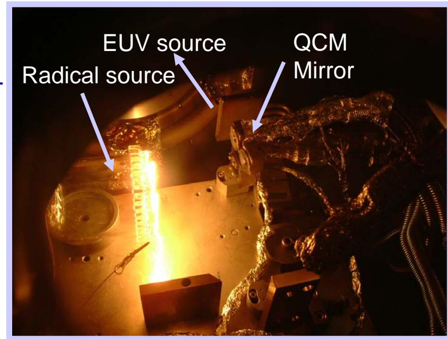
Sn thickness and cleaning rate were measured by QCM and normalized reflectance. Hydrogen radical density was more than  $10^{16}$  cm<sup>3</sup>.
