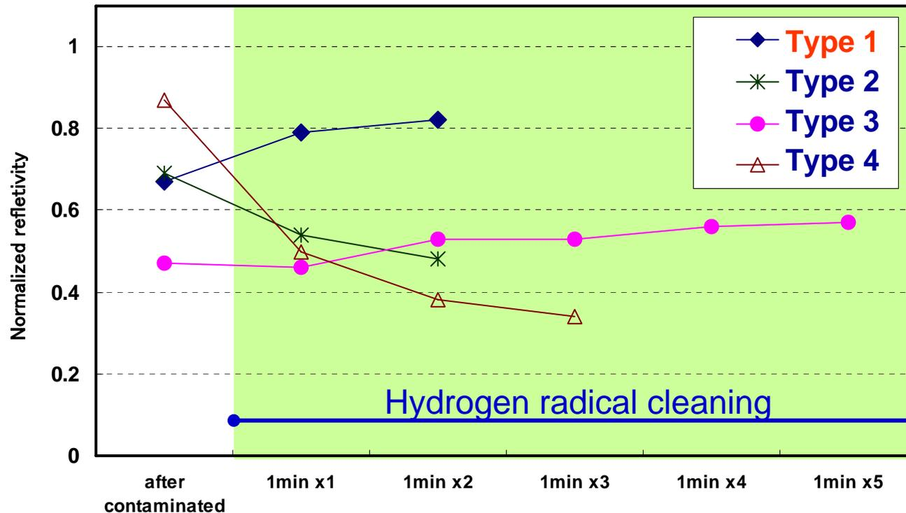
Debris of Sn contaminated the Sn-fueled discharge. Sample mirrors were different substrate and layer material. Reflectivity of the type No. 1 sample was improved by the cleaning.
