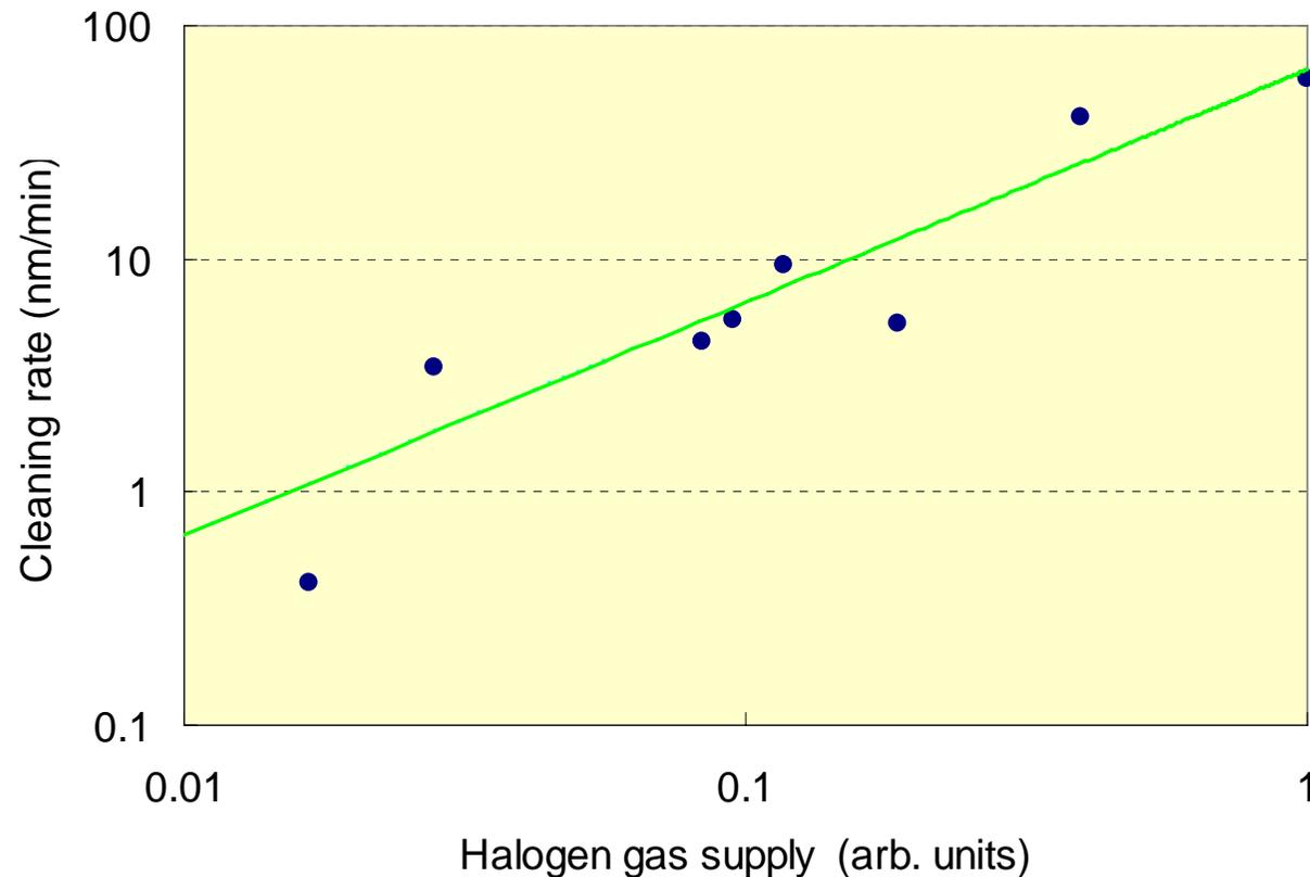
Cleaning rates of sample mirrors were sufficiently high. Possibly, the cleaning processing was enabled in a short time. The cleaning rate was calculated using cleaning time and layer thickness, before/after cleaning. The Sn thickness was measured by QCM or SEM.
