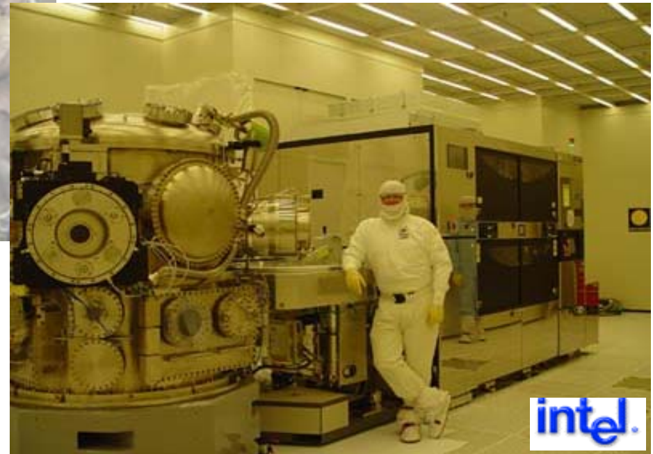
World's first commercial EUV lithography tool installed at Intel (Source: Intel)
