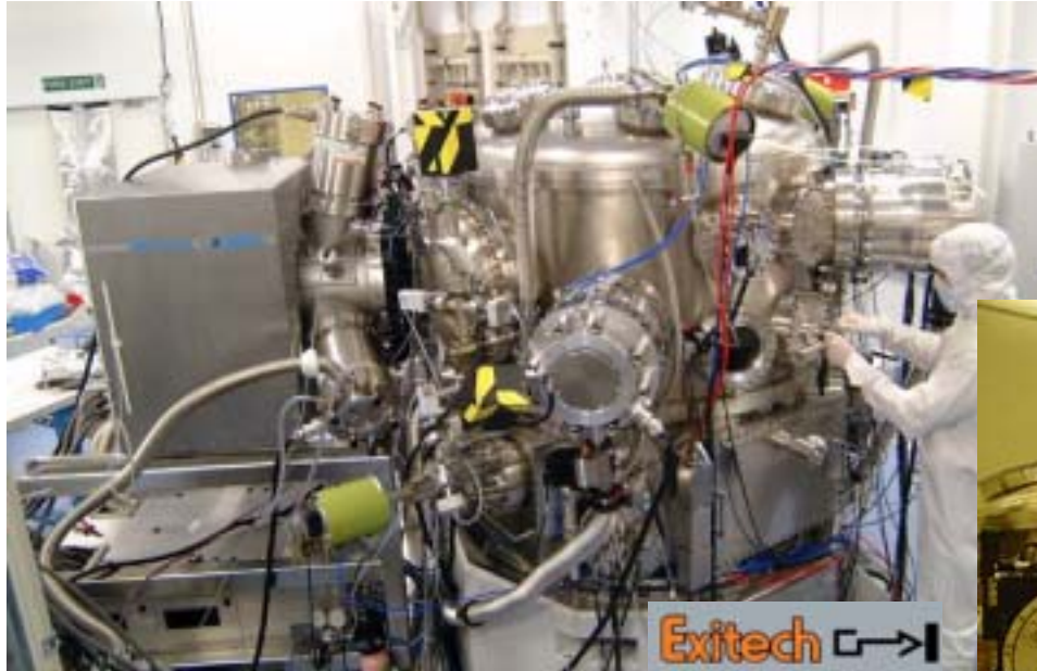
GDPP EUV source from XTREME technologies at microstepper at Exitech (Source: Exitech)
