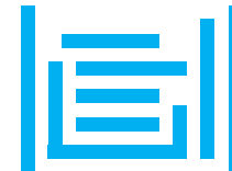
H&V Lines&Spaces Contact Hole array 18 nm half-pitch 18 nm half-pitch
