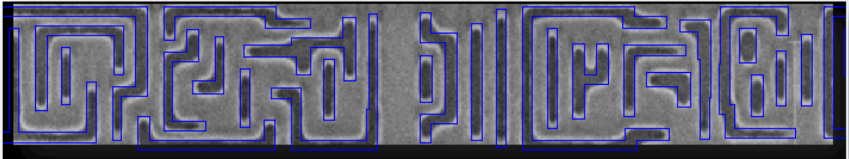
14nm node ARM M1 clip without OPC, 46nm minimum pitch, exposed on an NXE:3300B with conventional illumination
